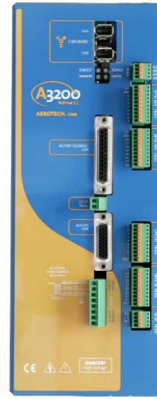
Ndrive CL Width: 103.7 mm Height: 265.2 mm
